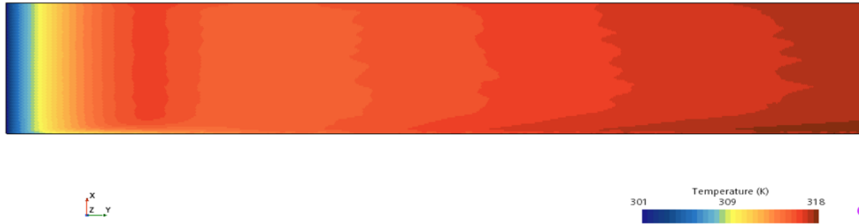
Figure 3.2: Contour along the smooth channel ( H = 7 mm and Re = 5000 )
